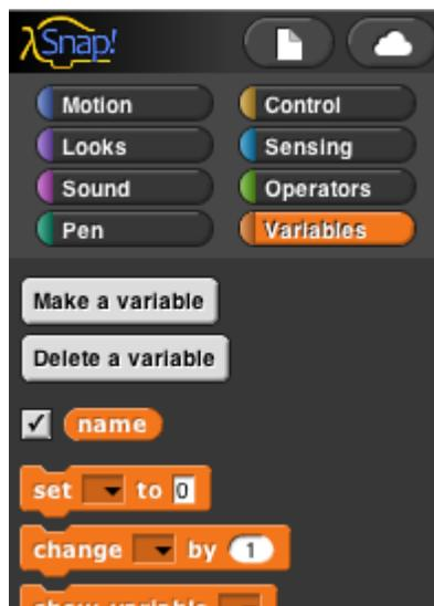
There's now a "Delete a variable" button, and there's an orange oval with the variable name in it, just like the orange oval in the **for** block. You can drag the variable into any script in the scripting area. Next to the oval is a checkbox, initially checked. When it's checked, you'll also see a *variable watcher* on the stage:
